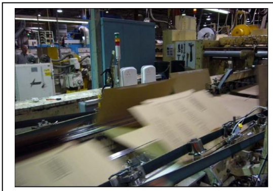
Figure 3: HIDE-Compliant RFID-Enabled Corrugated Cases Being Produced on a Flexo-Folder-Gluer at 900 fpm
