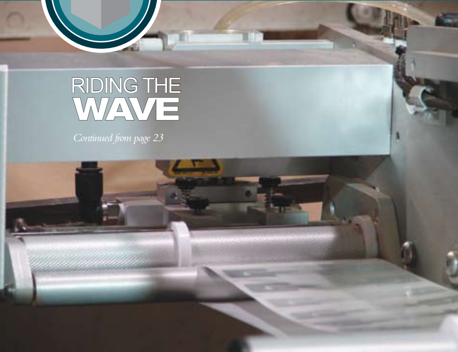
RFID inlays are being printed on a Label-Aire label printing-applicating machine at KruPak's LaSalle plant just prior to being embedded into a corrugated board sheet.
